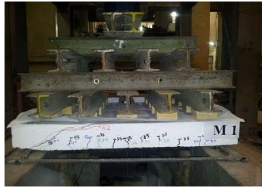
Figure 11: Shear cracks of specimen M1
