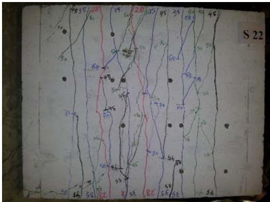
Figure 18: Cracks pattern of specimen S22
