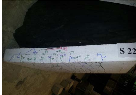
Figure 19: Shear cracks of specimen S22
