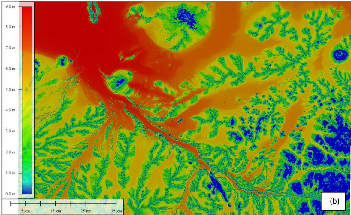
Figure 3: (a) SRTM 1''DEM and (b) Calculated MrVBF values resampled at 250m
