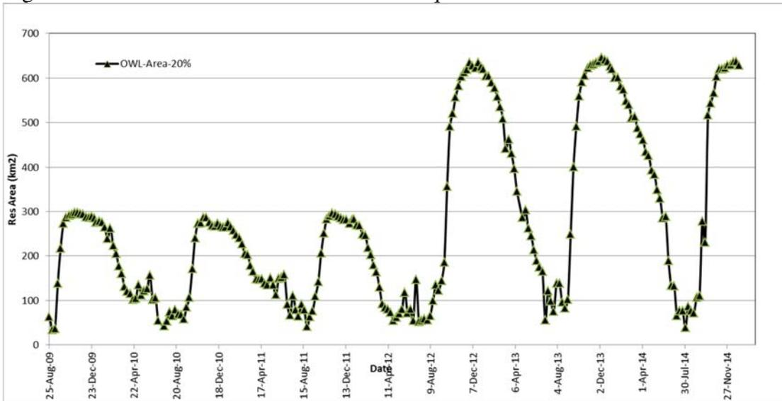
Figure 14: Extracted Reservoir Area from applying the new methodology using OWL threshold at 20% for the period from 2009-2014.
