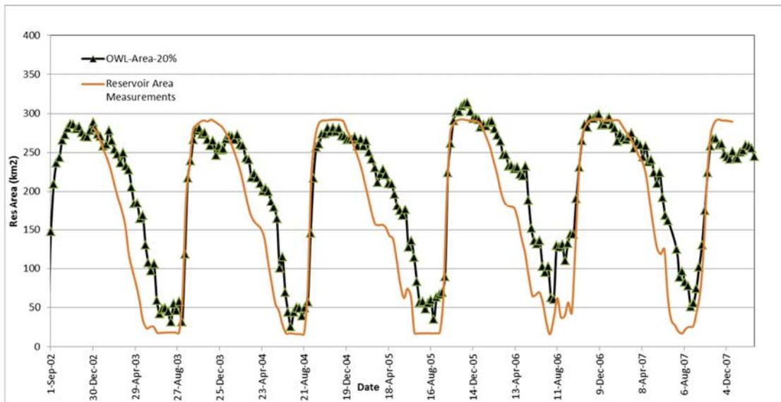
Figure 12: Comparison between Extracted Reservoir Area from applying the new methodology using OWL threshold at 20% and actual measurements for the period from 2003-2007.
